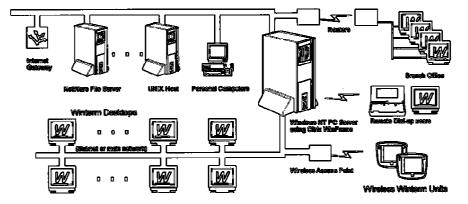
Winterm wireless thin clients expand on the extensive connectivity options already available for Winterm 2000 series thin clients. Wireless Access points provide connection to 10Base2 or 10BaseT corporate networks and provide access for multiple Winterm 2930 terminals.
