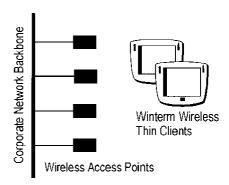
Multiple access points can be used to wire a complete building or site. Winterm Wireless thin clients automatically hop between access points to provide seamless connectivity to users wherever their jobs take them.
